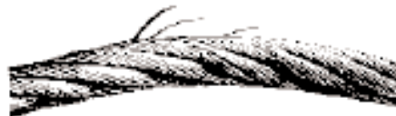
Wire Rope Fatigue Failure
