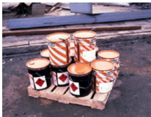
Flammable materials stored in fire-resistant containers.
