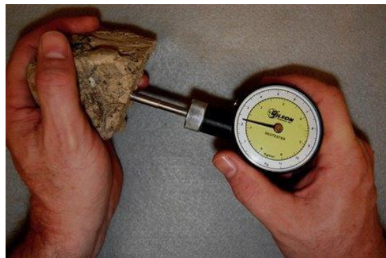
Figure 3.4.1.3. Testing with a penetrometer.
