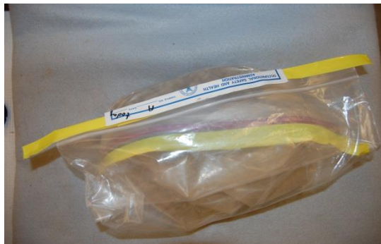
Figure 2.3. A properly packaged, sealed, and labeled excavation sample.
