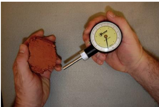
Figure 3.4.1.2. Flat face of sample ready for testing.
